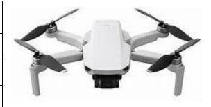
**Description:** This is a battery powered, remotely operated Unmanned Aerial System (UAS) that is able to record video and audio with approximately 30 minutes of flight time. The DJI Mavic Mini is designed to be operated within sight of the operator or a spotter. Each aircraft is equipped with a camera capable of relaying a real-time image back to the operator.
